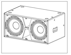
The 10" low frequency transducers are equipped with waterproof cones and this feature, together with the moisture resistant cabinet, makes the SW210P suitable for use in light duty outdoor applications. The transducer technology combines a 3" sandwich voice coil with a fiberglass former progressive wave Konex spider; a cloth surround with DAR technology; a high excursion ferrite magnet circuit with demodulating ring; and a ventilated voice coil and magnet to reduce power compression.
